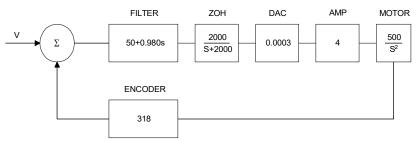
Figure 10.6: Mathematical model of the control system
