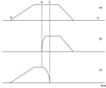
Figure A.10: Vector and Axes Velocities
