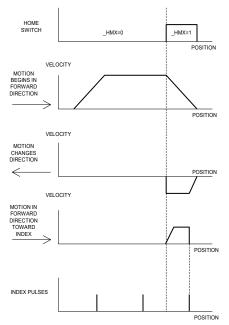
Figure 6.22: Homing Sequence for Normally Closed Switch and CN,-1
