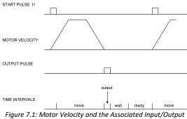
Figure 7.1: Motor Velocity and the Associated Input/Output signals
