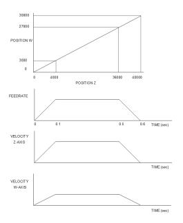
Figure 6.6: Linear Interpolation
