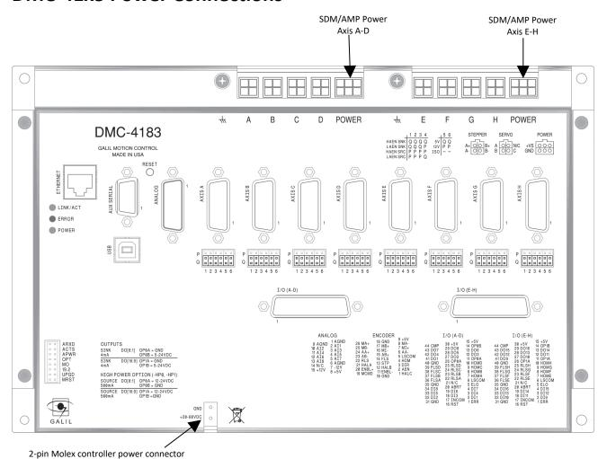
Figure 2.5: Power Connector locations for the DMC-41x3
