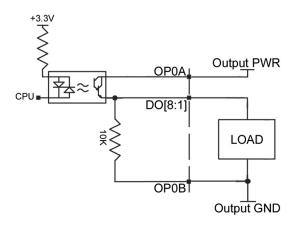
Figure 3.10: 25mA sourcing wiring diagram for Bank 0, DO[8:1]
