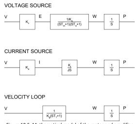
Figure 10.5: Mathematical model of the motor and amplifier in three operational modes
