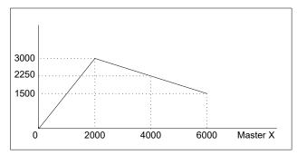
Figure 6.13: Electronic Cam Example
