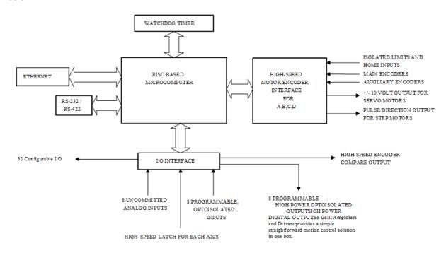
Figure 1.4: DMC-41x3 Functional Elements
