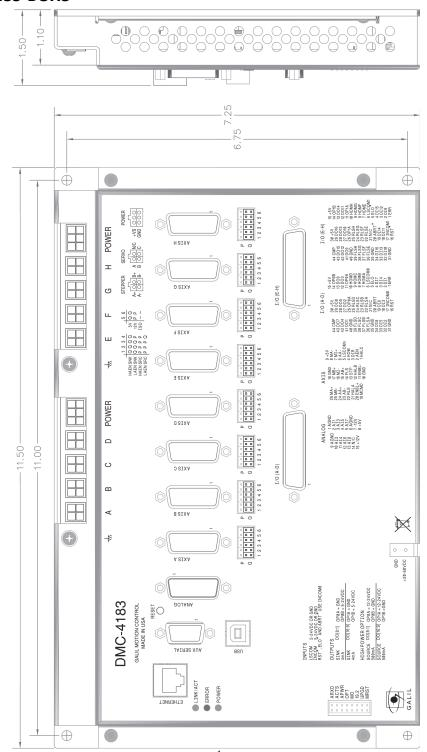
Figure 2.4: DMC-41x3-BOX4 Dimensions  $^{1}$  (in inches) where x= 5, 6, 7, and 8-axis
