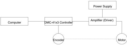
Figure 1.5: Elements of Servo Systems
