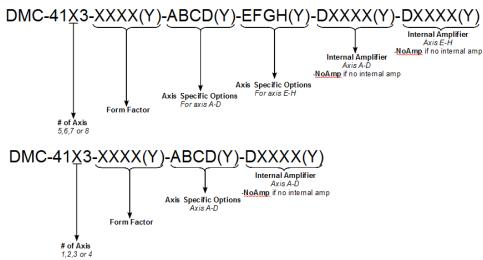
Figure 1.3: Layout of the full DMC-41x3 part number
