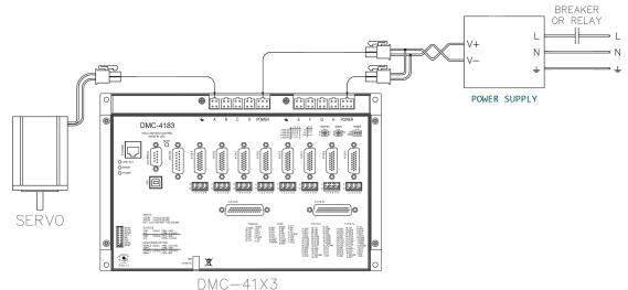
Figure 2.7: Wiring for DMC-4183 with Amplifiers
