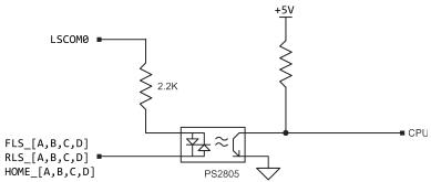
Figure 3.3: Limit Switch Inputs for Axes A-D
