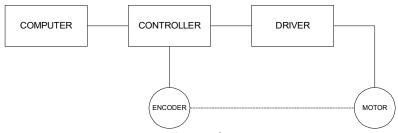
Figure 10.1: Elements of Servo Systems
