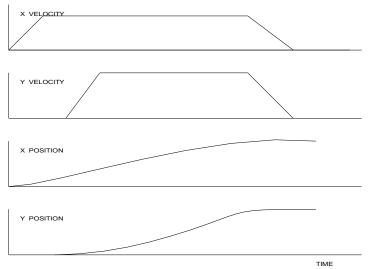
Figure 10.2: Velocity and Position Profiles
