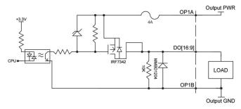
Figure 3.13: 500mA sourcing wiring diagram for Bank 1, DO[16:9]
