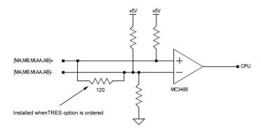
Figure A.1: Encoder Inputs with -TRES option
