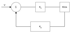
Figure 10.4: Elements of velocity loops
