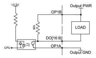
Figure 3.9: 25mA sinking wiring diagram for Bank 1, DO[16:9]
