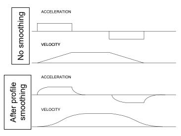
Figure 6.21: Trapezoidal velocity and smooth velocity profiles
